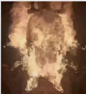
ASTM F1930-23 Standard Test Method for Evaluation of Flame-Resistant Clothing for Protection Against Fire Simulations Using an Instrumented Manikin
